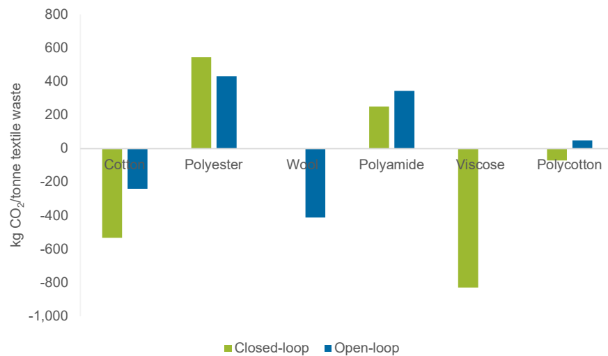
Figure 9. Results of environmental assessment of mechanical recycling processes for textile fibres (Huygens et al., 2023)
